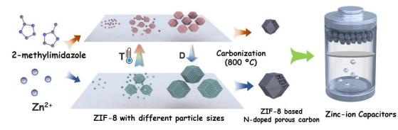
**Graphical abstract 4).** A schematic illustration of the size dependent effect of ZIF-8 in nanocarbon based zinc-ion capacitor (ZICs).
