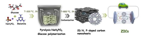
**Graphical abstract 5).** Schematic diagram for the N, P co-doped 2D carbon nanosheets by a gas-steamed method for high performance zinc-ion capacitor.
