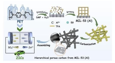
**Graphical abstract 3).** The schematic illustrating the directly recycling waste Polyethylene terephthalate (PET) bottles into MIL-53(AI) for the synthesis of accordion-like porous carbon and its application as high-performance zinc-ion capacitor (ZICs).
