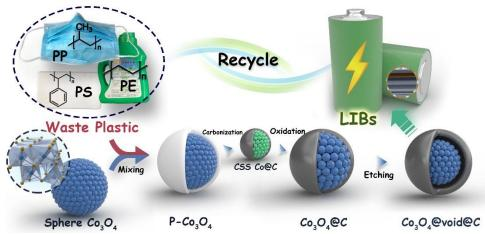
**Graphical abstract 1).** The schematic illustration of the recycle the real-world waste plastics into Co<sub>3</sub>O<sub>4</sub>@void@C composites for lithium-ion batteries (LIBs).
