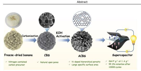
**Graphical abstract 6).** The preparation process for the synthesis route of 3D N-doped porous carbon materials for supercapacitor.
