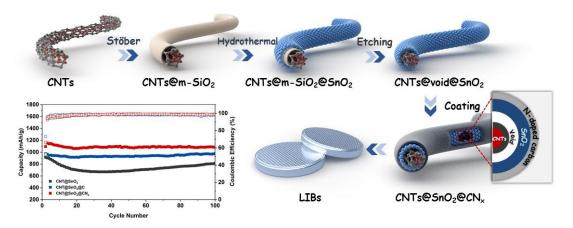
**Graphical abstract 2).** The fabrication scheme of N-doped carbon coated CNT@SnO<sub>2</sub> sword-sheath structures for lithium-ion batteries (LIBs).
