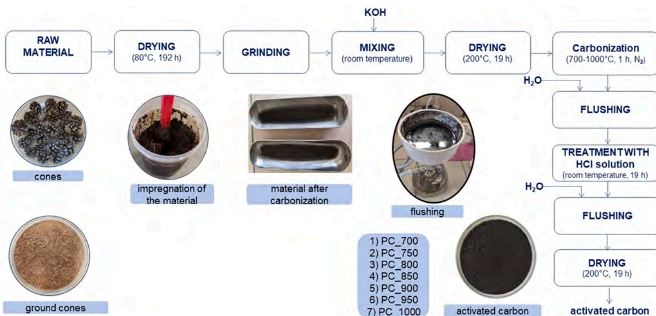
Fig. 2. Simplified block diagram for preparing carbon catalysts from pine cones.
