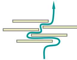
Figure 8.1: A good filler dispersion leads to a tortuous path, which impede fluid permeation.
