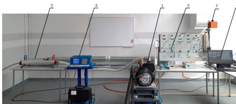
Figure 2. Scheme of the test stand: 1 — diesel engine; 2 — fuel tank; 3 — measuring devices; 4 — computer; 5 — calorimeter; 6 — exhaust gas analyzer.
